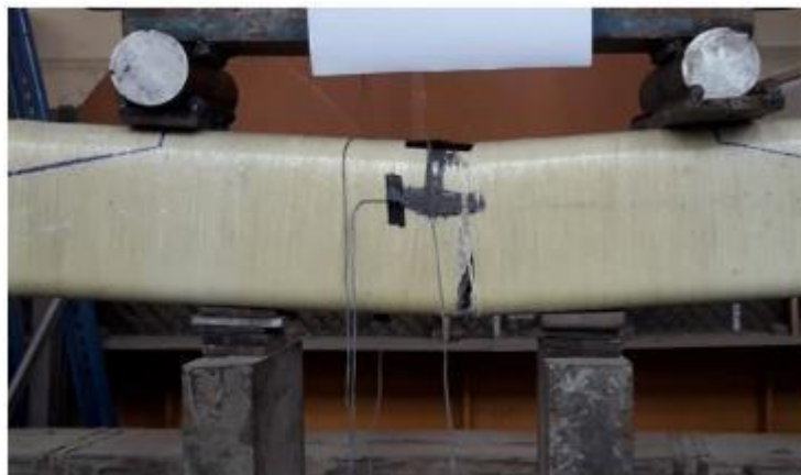
Fig. 5: Tension Failure pattern on bottom flange
