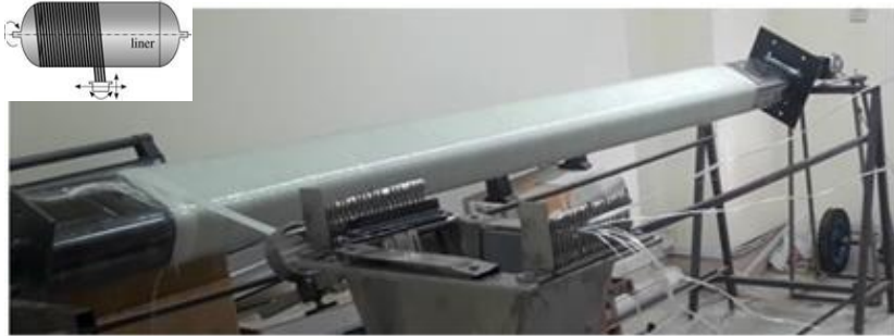
Fig. 1: Circumferential pattern of winding [90°]
